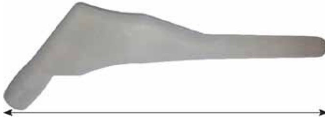
Figure 3. Prototype of injection moulded hip stem
